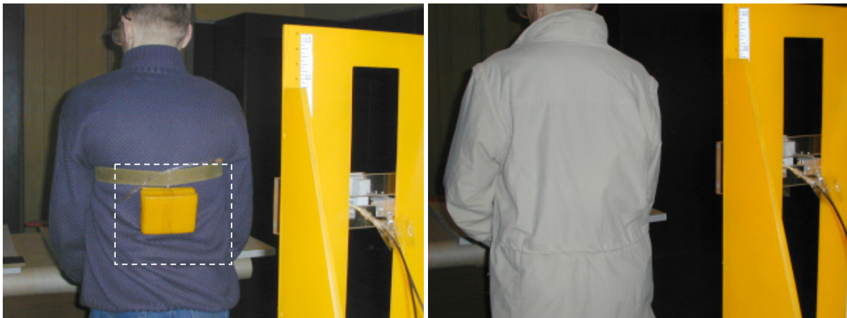
Figure 2. Experimental setup with two antennae. A “suicide bomb” was simulated by wax attached to the body and covered by a raincoat.
